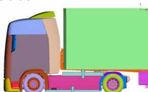
Figure 5-3 Active side skirt Extension for the truck
