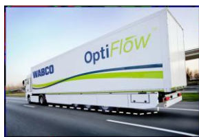
Figure 5-10 Active side skirt extensions for the trailer
