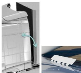
Figure 5-2 Active air deflectors for the truck
