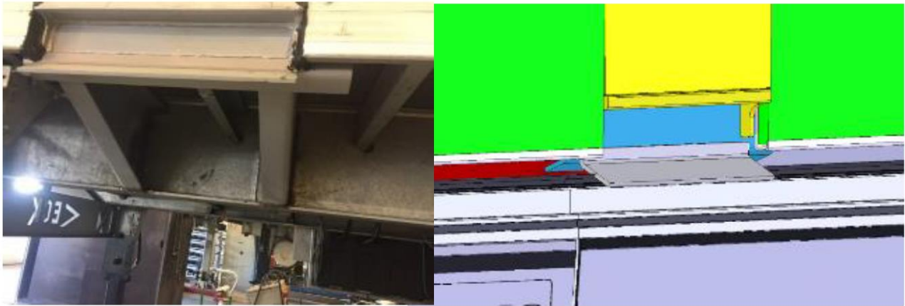
Figure 13. Pockets welded in the chassis with push out strip
