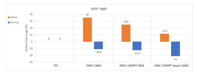
The concept can mitigate the increased fuel consumption of EMS1 vehicles by 19.5% - 23.6% depending on the leg of the use case. The transport efficiency gains can be improved up to 29%.
