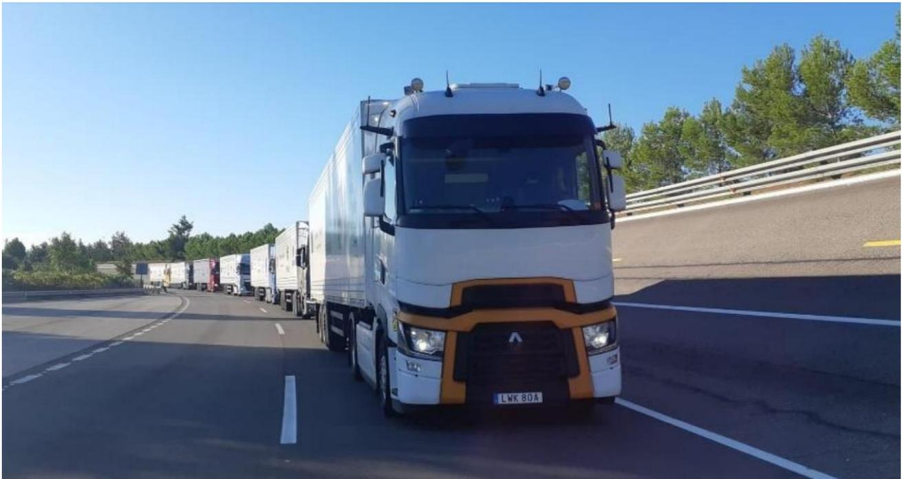
Figure 10. The multi-brand platoon with seven trucks demonstrated during the ENSEMBLE project
