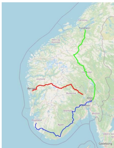
Figure 6-5: Train routes used for validation of energy consumption by Energy module: Route in red: Bergen-Alnabru (362.7 km), Route in blue Sandnes-Alnabru (571.7 km) and Route in Green Trondheim-Alnabru (554.8 km)
