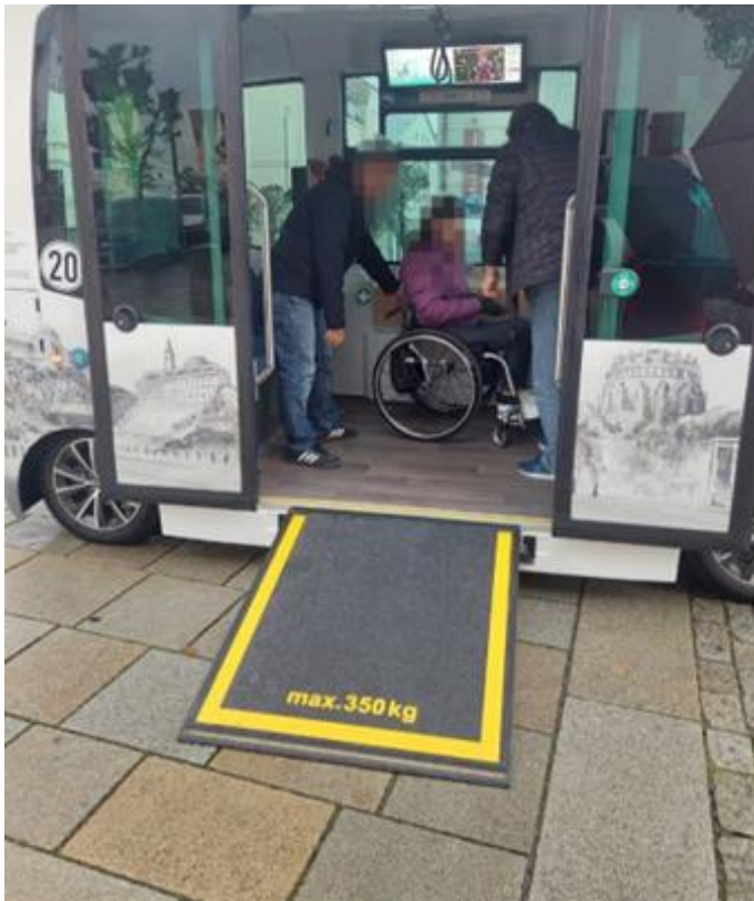
Figure 23: Extended ramp at a bus stop without sidewalk (much steeper!)
