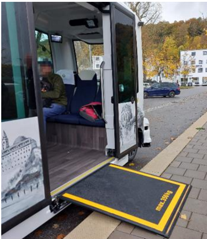
Figure 22: Extended ramp at a bus stop with sidewalk
