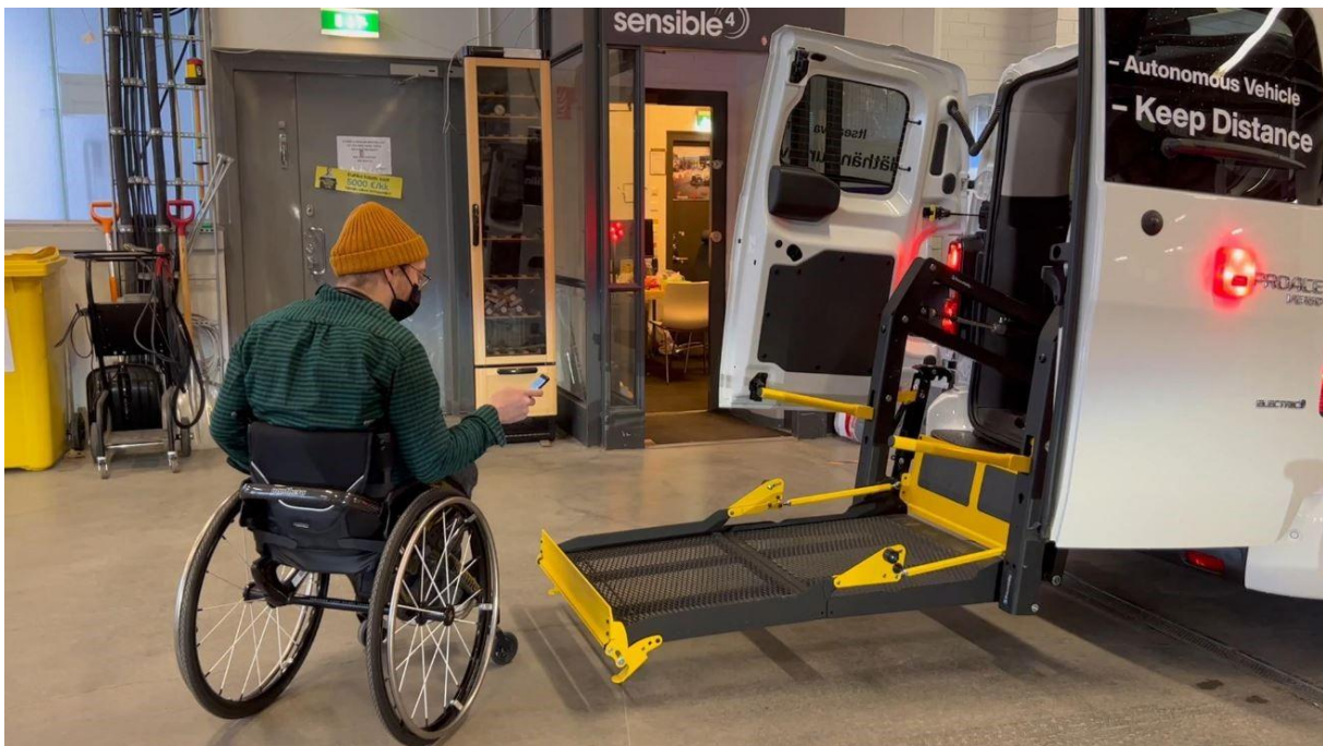
Figure 39: Testing of an app-operated wheelchair ramp.
