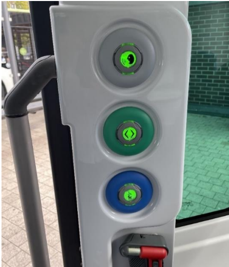
Figure 5: Mechanical Control Buttons Grey Customer Service Green Door Blue Ramp
