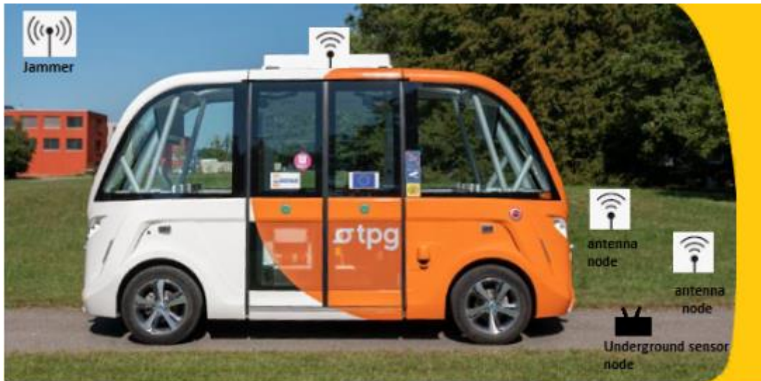
Figure 3: The Jammer node interferes with the shuttle antenna node and the (above-the-ground) transceiver antenna nodes. An underground sensor node is added in order to manipulate the Jammer Transition matrix and therefore its Equilibrium State Distribution. The underground node is not affected by the jammer and can be connected underground with whichever supporting transceiver antennas that we choose.
