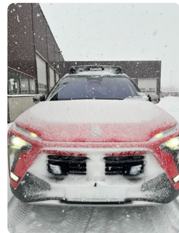
Figure 66: Snow covering sensors
