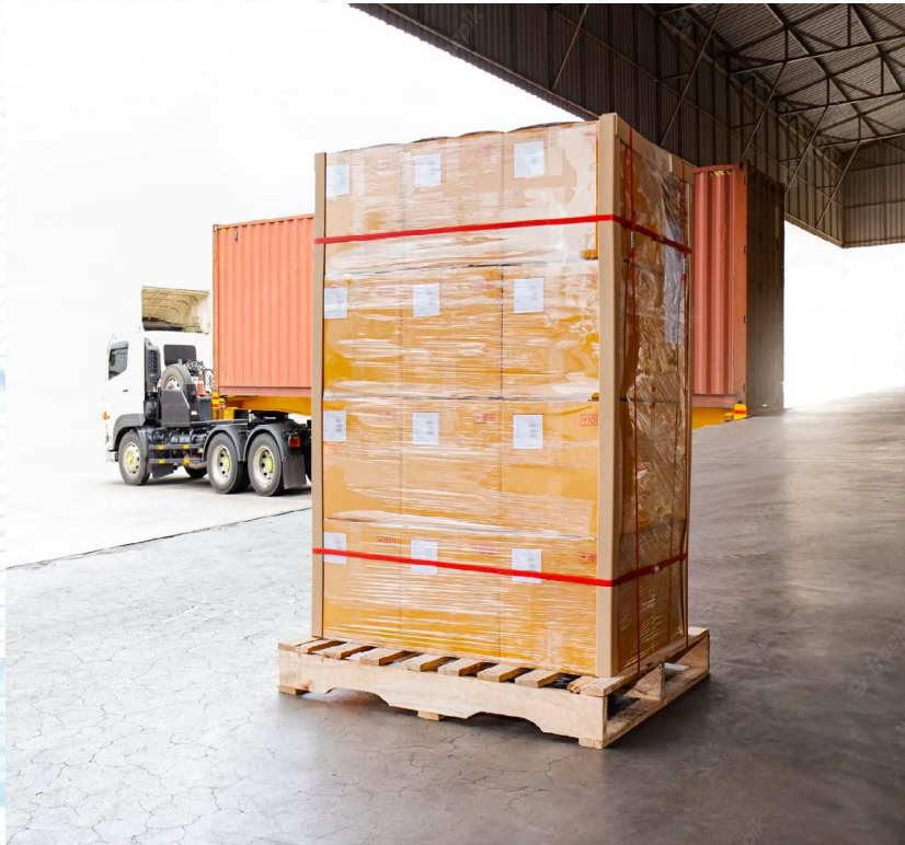
Example of an actual standard pallet: cardboard, pallet edges, plastic film, area utilisation of the pallet not optimised...!
