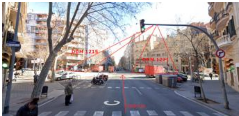
Figure 33 Positioning of cameras in Valencia street overlooking chamfered spaces
