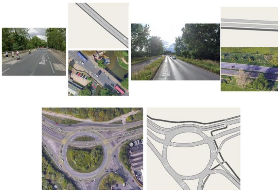
Figure 37 I) Cycle lanes right and left from road; II) Bidirectional cycle track left of road; III) Junction Crossings
