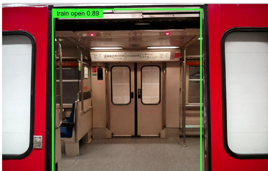
Figure 20: Door opening detection (2/4)
