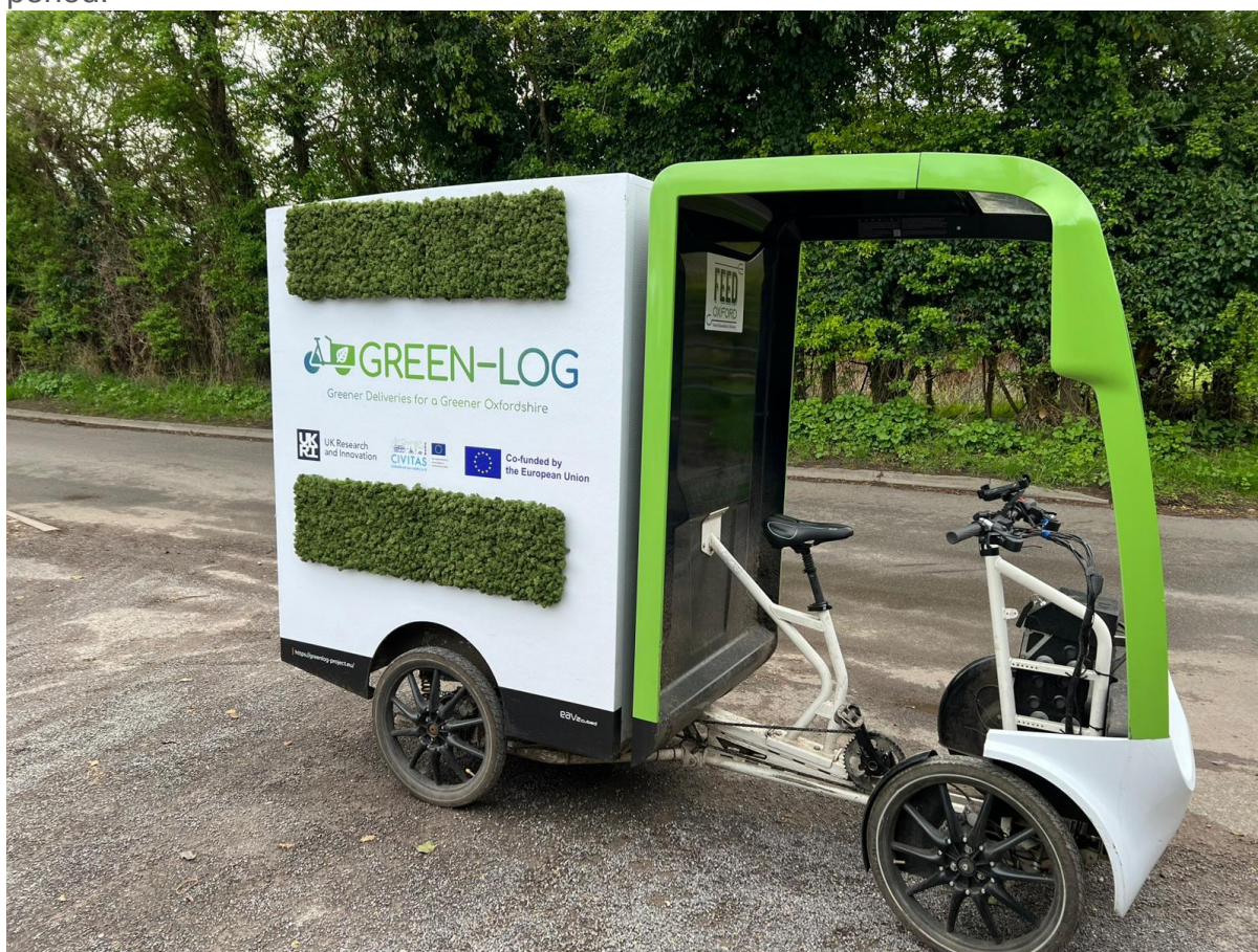
Figure 45 The Mobile Delivery Hub, and EAV 4 wheel cargo bike that will be converted into a self driving vehicle.
