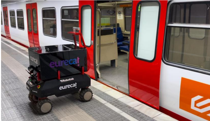
Figure 21: Door opening detection (3/4)
