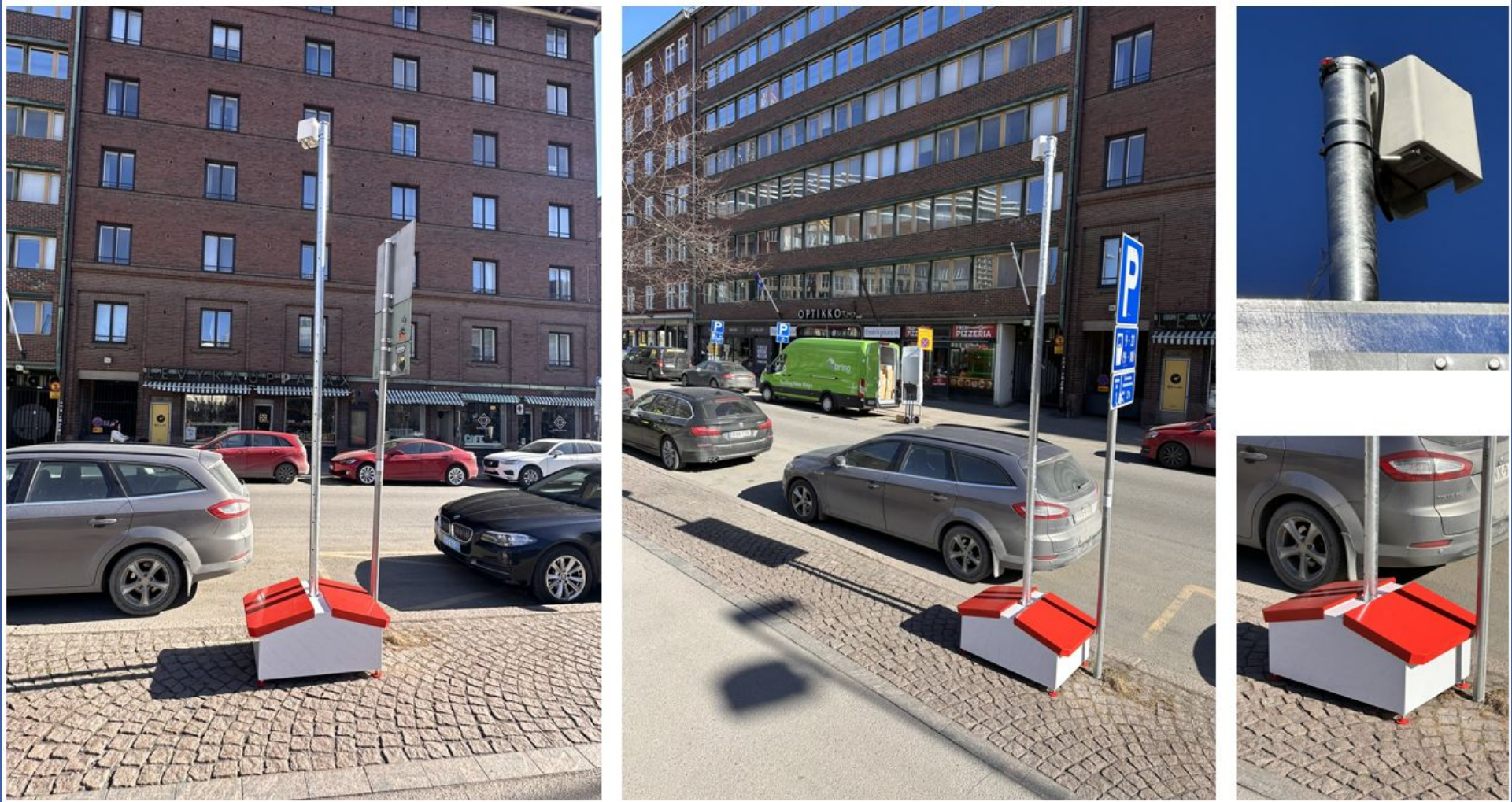
Figure 17. FlowCube stand-alone data collection system with small footprint installed in a street environment
