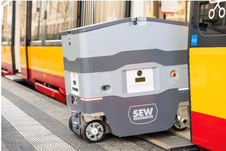
FIGURE 15: DELIVERY ROBOT ENTERING TRAM OVERCOMING STEPS AND GAPS
