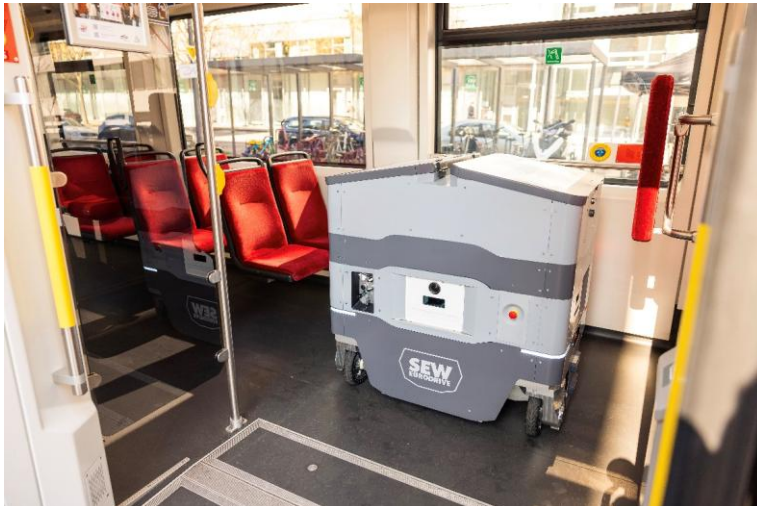
FIGURE 16: DELIVERY ROBOT IN MULTIPURPOSE SPACE WITHIN TRAM – HIGH MANEUVERABILITY BY OMNIDIRECTIONAL CHASSIS (HERE: LATERAL DRIVING)
