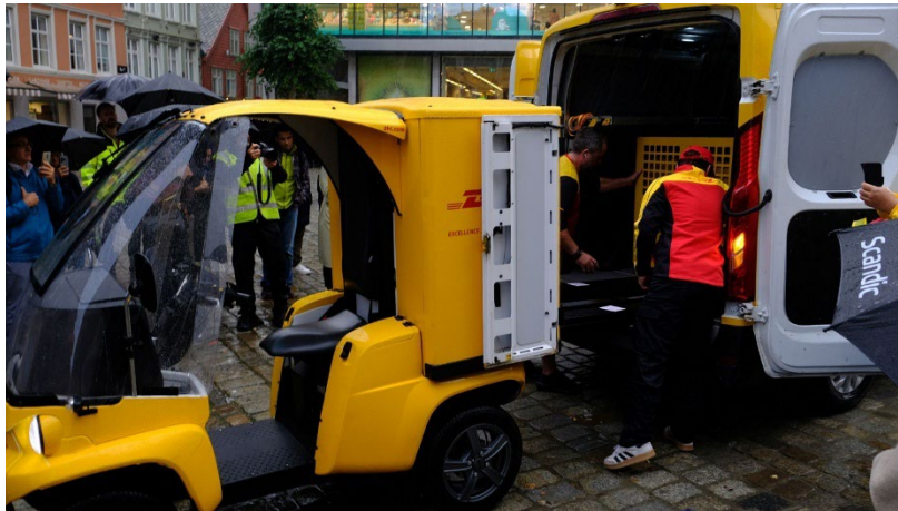
Figure 2. Illustration of a standardized cargo type, the Swapbox (Paxster, 2025).
