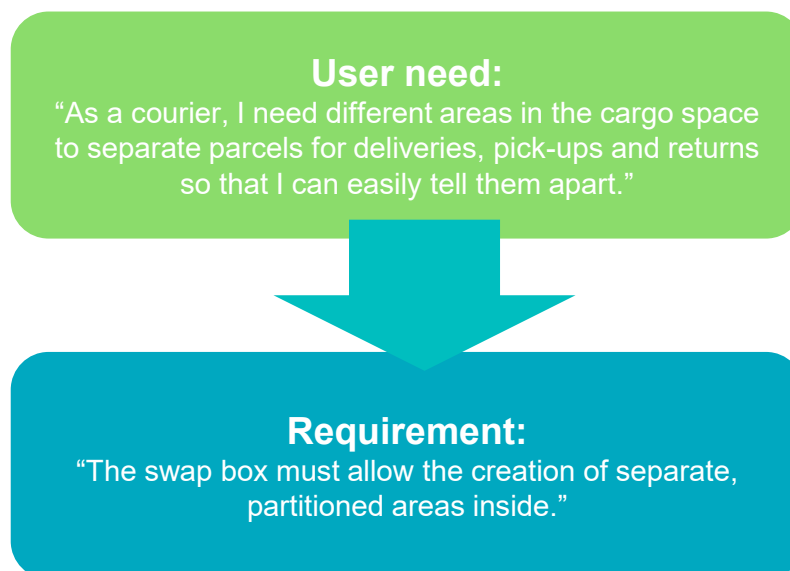
Figure 6. Procedure for transition from user needs to requirements on an example from swap box
