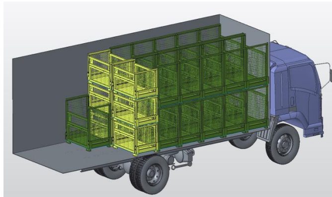
Figure 10. Improved stackability of foldable PI grid boxes
