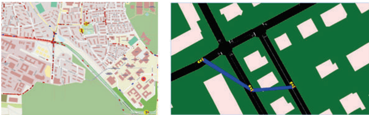
Figure 42. Simulation framework with Veins-Omnet
