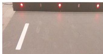
The cost of installation and maintenance would be reduced if studs were installed less densely. In the examples shown on the left alongside, studs were installed at 0.5m frequency. Next, alternate studs were switched off, to simulate a 1.0 metre spacing, and participants were asked if they thought that this would be sufficient.
