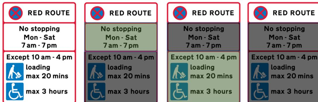
This set of signs was designed to obtain reactions to the possibility of highlighting the regulations that applied at a specific time of day, on LED signs (grey = not applicable).
