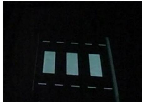
The lighting of the zebra markings was then lowered and raised, with the suggestion that the lights would be intensified when a pedestrian approached the crossing, to alert drivers to their presence.
