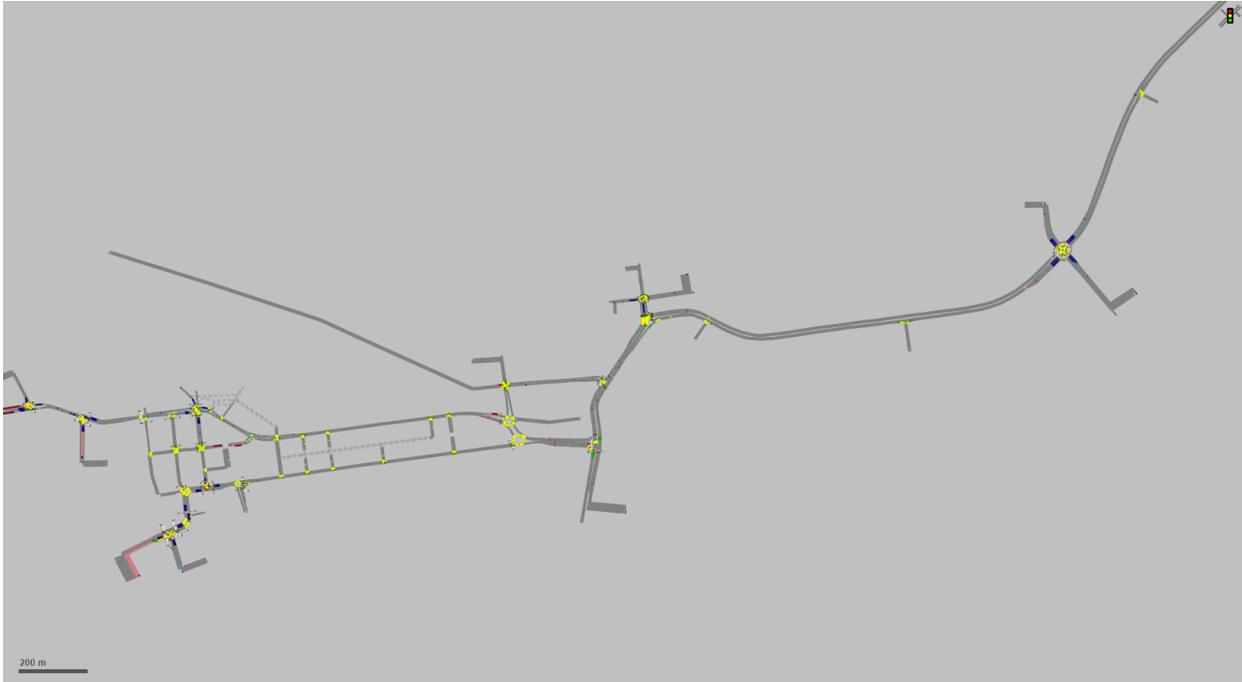
**Figure 8:** VISSIM simulation network of the Malmö corridor
