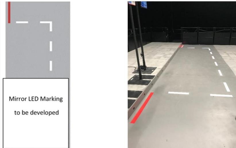
Under normal and strong lighting conditions, the LED and painted lines were largely indistinguishable, but under low lighting conditions the LED markings were much brighter and clearer.
