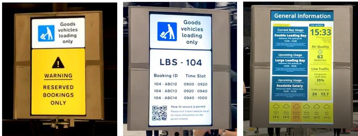
Drivers were shown an experimental three-sided LED sign, under development by Grid Smarter City, to be used in conjunction with their dynamic loading booking system. The first sign face warns drivers that this section of the kerbside is reserved for drivers with bookings only. The second face records details of each booking (i.e., booking reference and time slot booked), while the third face is used for public service information, such as weather conditions, or local public events.
