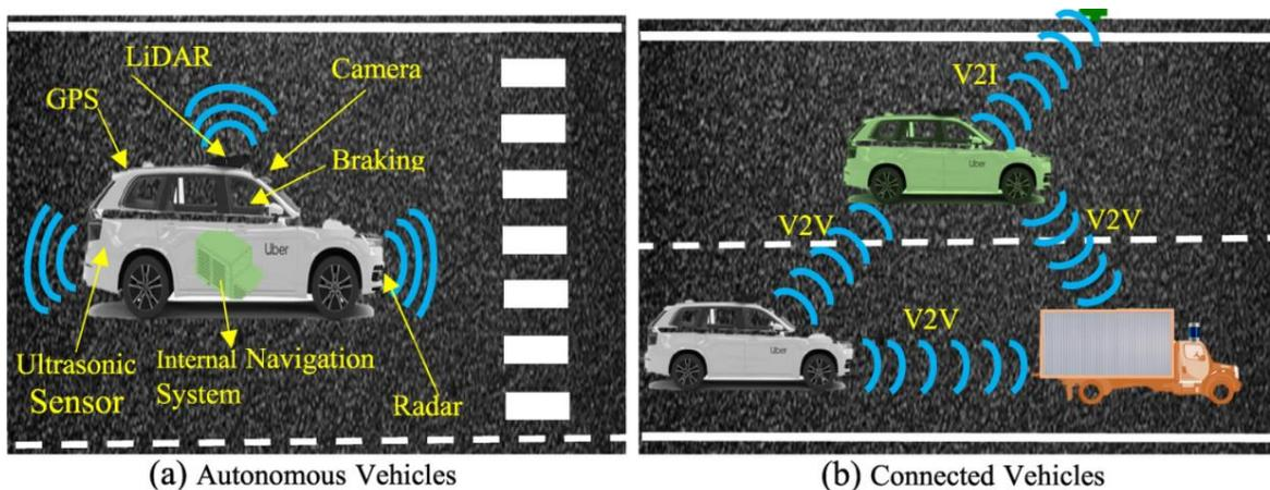
**Figure 1:** Autonomous vehicle and Connected vehicle [source [2]]
