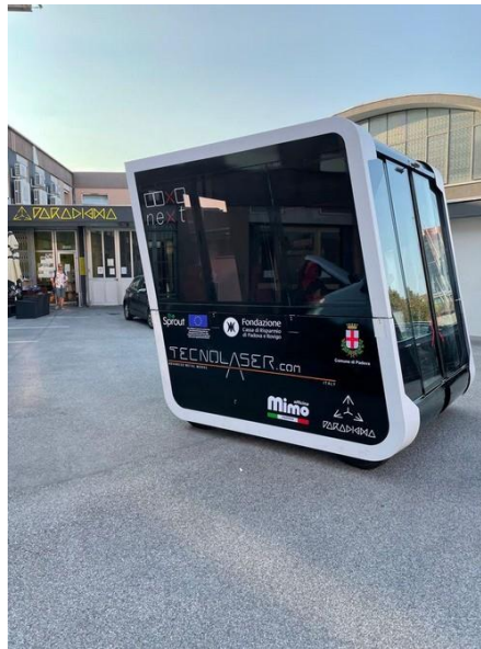
Figure 1. The NEXT system: modular pod for passengers and cargo-hitching.
