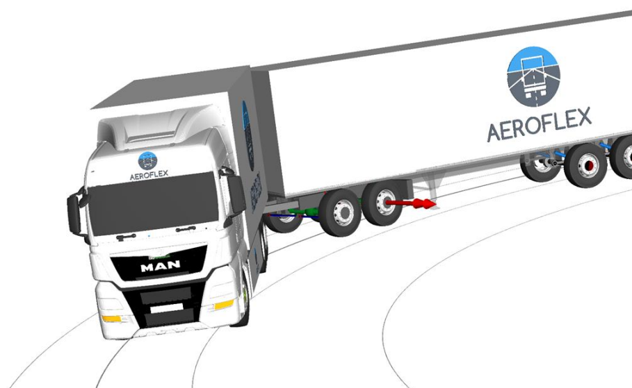
Figure 11 Detailed vehicle model of EMS1 vehicle combination in a cornering scenario
