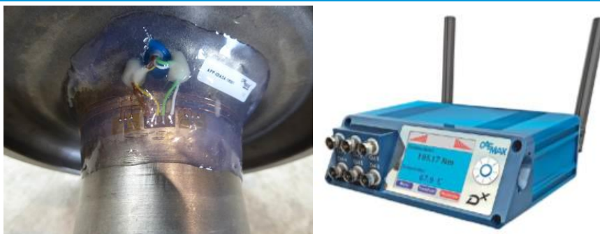
Figure 28. Strain gauges on half shafts and telemetry system
