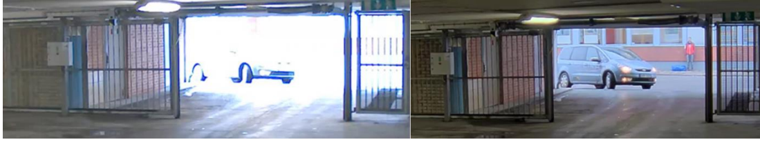
Figure 9: Difference between a non WDR (left) and a WDR camera (right)
